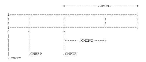
These byte pointers and other information are contained in a command state block whose address is given as an argument to the COMND monitor call. The .CMINI function initializes these pointers.
