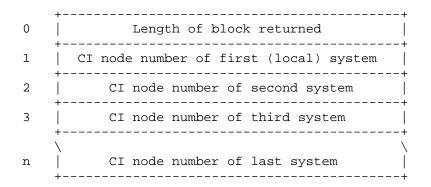
1 .INCFG This function causes the CNFIG% monitor call to be executed on the specified system. See the CNFIG% monitor call for more information.
